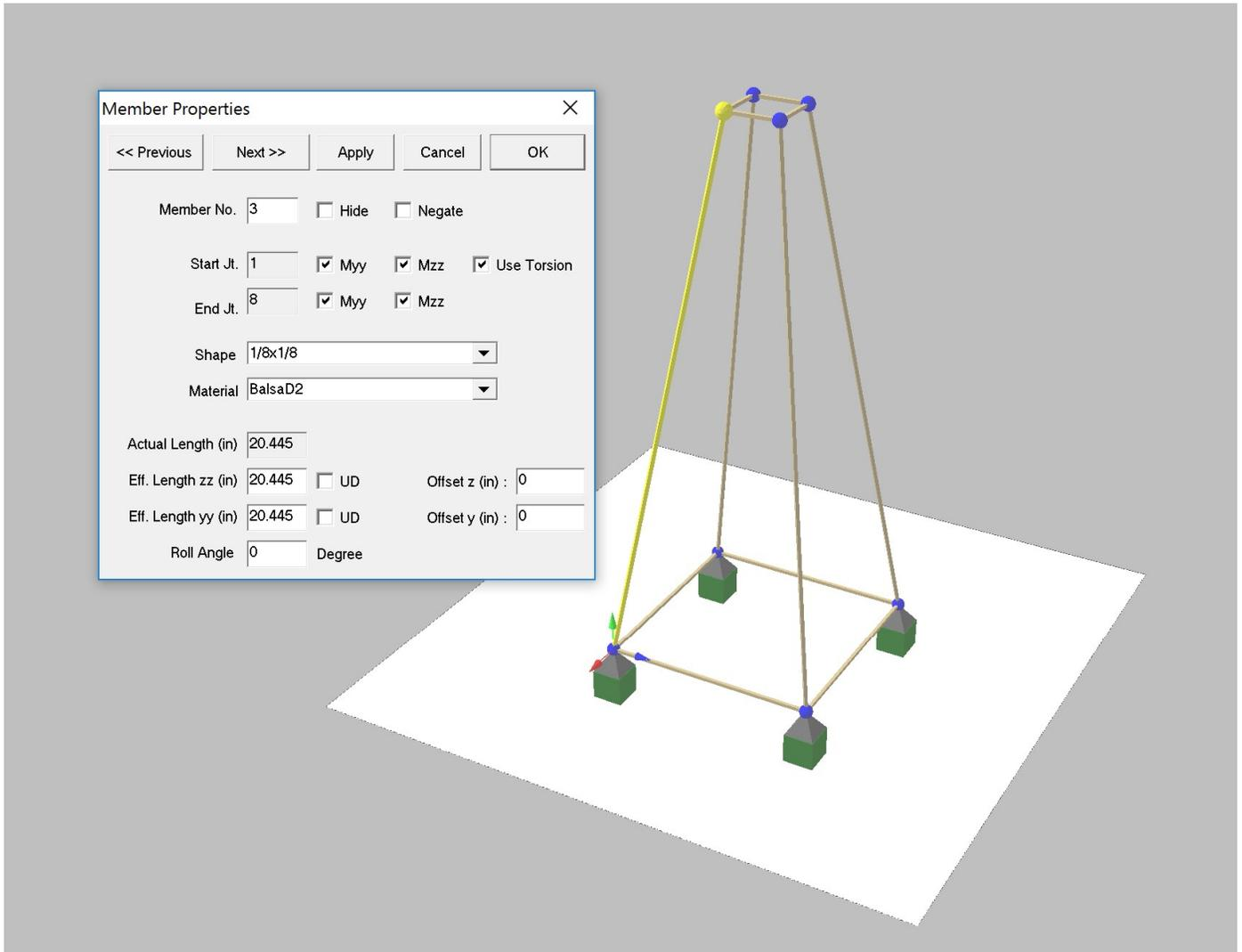
This example uses a unit vector to locate a node 4" from the base of the column measured along the column.
