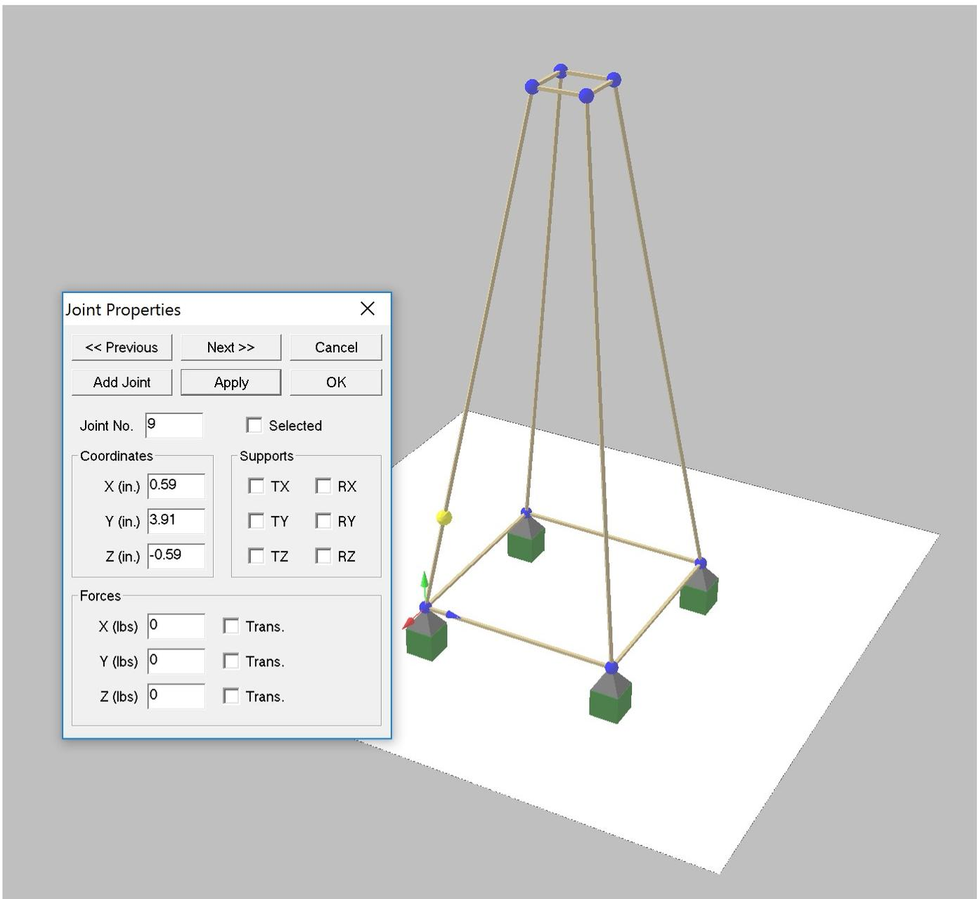
Select "Properties" from the Joints menu. Click the "Add Joint" button and change the coordinates of the new joint to .59, 3.91, -.59 then click "Apply". Mathmagic!
